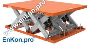
NomenclatureModel LSH 20Product Type:Lift Scissor HydraulicLift Style:20CCapacity:400 = 40000 lbsRaised Height:87"Platform Size:96" width × 216" length
