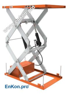
Employing an internal power unit that supports a variety of voltages (120, 208, 220, and even 480) the LSH015 Hydraulic Scissor Lift Table offers a profile as low as 7", and a raised height of between 43" and 70." With a formed upper and lower frame, this two cylinder lift raises from 500 to 2500 lbs., with either 36" or 57" of travel. This lift is available in two platform sizes, either 18" by 36" or 32" by 50".
