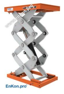
High strength steel supports 55" of travel up to an 80" raised height with the LSH13 Hydraulic Scissor Lift Table. This powerhouse lift has a lowered height of 25", and the capability of lifting up to 20,000 lbs. The 32" by 54" platform can be supported by the optional ratchet system, and employs scissors designed specifically to support stable upward movement.
