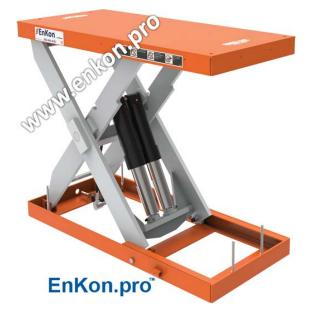
A popular option for general industry use, the LSH01 Hydraulic Scissor Lift Table provides a welded construction top and bottom frame along with many safety features. Available with lift capacities ranging from 500 to 4000 lbs., the LSH01 has several travel options, from 24" to 60." The rectangular platforms range from 17" to 24" wide and 42" through 88" long.
