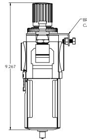
BRACKET DESIGNED TO ATTACH TO PEDESTAL, CAN ALSO BE USED FOR CUSTOM MOUNTING
