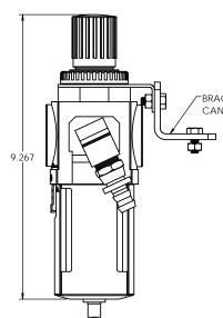
BRACKET DESIGNED TO ATTACH TO FOOT PEDAL ENCLOSURE, CAN ALSO BE USED FOR CUSTOM MOUNTING
