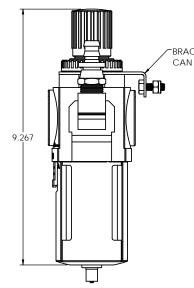
BRACKET DESIGNED TO ATTACH TO PEDESTAL, CAN ALSO BE USED FOR CUSTOM MOUNTING
