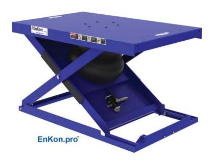
With a raised height of up to 36", the Enkon LSA12 Pneumatic Scissor Lift Table offers 31" travel with a high capacity of up to 6000 lbs. The  $37" \times 63"$  platform is teamed with a 5" profile, and the lift utilizes the airbag and the mechanical advantage of the scissor to offer great lifting power in a lift that weighs under a thousand pounds.
