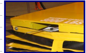
Cart present switch: Lift will not raise unless switch is activated
