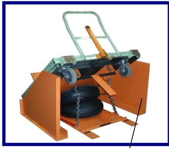
Guides located on outside of system positioner, floor
